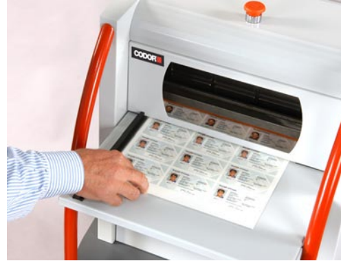
2. The input sheet positioned against the X-Y ledge.
