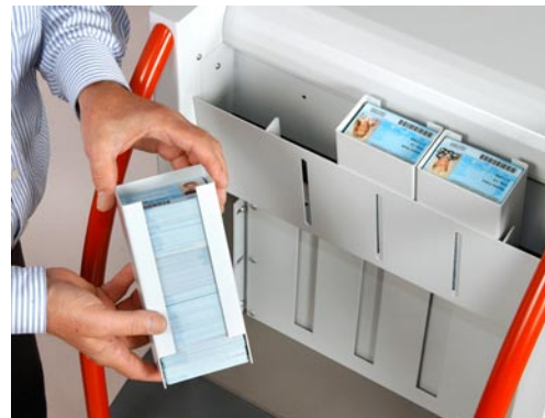
6. Stacker capacity depends on final card thickness.
