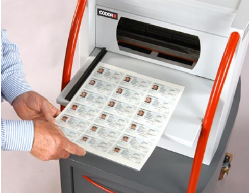
1. The input sheet is easily inserted into the cutter.
